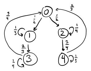
and then by using the Markov property to show that that the length of any sample path going from 0 to 0 must be the sum of some (independent) geometric random variables.
