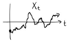
We have already seen (via scaling limits) that an OU process is mean-reverting since it is a limit of AR(1) processes that by definition are mean-reverting. But this SDE formulation gives us another reason why it mean-reverting: It has drift function  $\mu(x) = -\theta x$  which means the average velocity points to state 0, and the strength of the velocity increases when  $X_t$  is far away.
