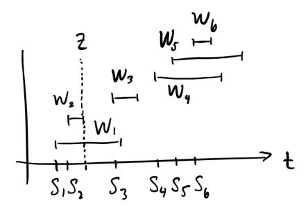
Here, the vertical axis does not mean anything in particular; we just use the vertical spacing to separate the horizontal bars representing the processing times.
