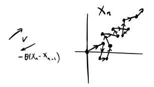
Here, we think of v as "velocity" and  $\theta$  as the "drag coefficient". This means that the motion is slowed by applying a force which acts opposite to the direction of motion.
